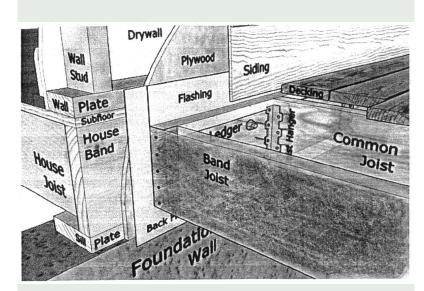
Flashing shall be between bands for full depth and kick out underneath if siding below. Flashing shall extend underneath siding above a minimum 2". Aluminum flashing shall not be used.
