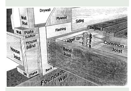
Flashing shall be between bands for full depth and kick out underneath if siding below. Flashing shall extend underneath siding above a minimum 2". Aluminum flashing shall not be used.
