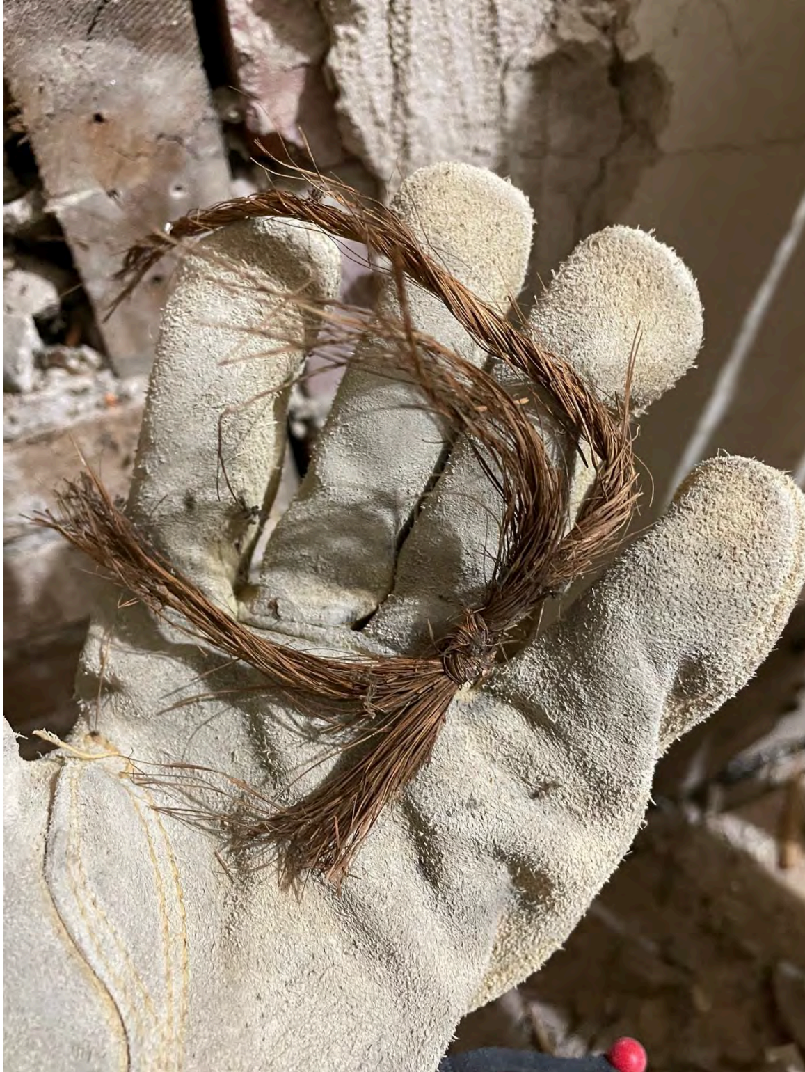
Figure 24 Artifact Braided Horse Hair Found in Failing Plaster Walls. Horse Hair Originally Used to Strengthen the Plaster Creating a Fibrous Network for the Material to Adhere to. Modern Methods Include the Addition of Fiberglass or Similar Material.
